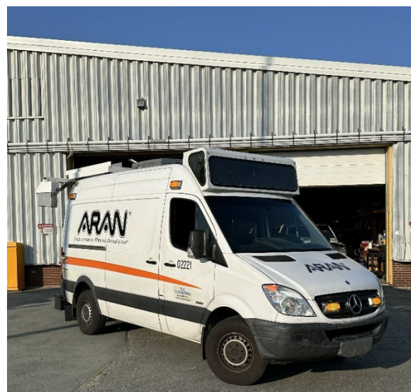
Automatic Road Analyzer (ARAN) (Office of the Auditor General of Nova Scotia photo)
